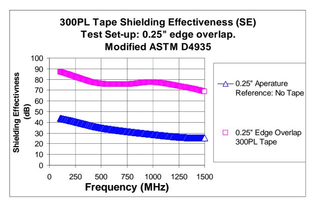
EMI Shielding performance can vary depending on several factors, including items such as test method, edge overlap of 3M<sup>TM</sup> Aluminum Foil Tape 300PL as it covers a gap or aperture opening, geometric shape, and application details of 3M tape 300PL.
