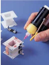
Lightweight, reliable EFD hand-lever valves solve many difficult assembly fluid applications, where controlled beads of cyanoacrylates, anaerobics, adhesives, grease, MEK, paint-based inks, solder masks and glues are applied.
