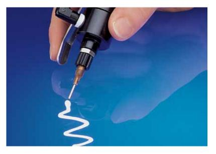
To get the best deposit control, select the most appropriate outlet tip. Each dispense hand valve includes a selection of tips. A wide variety of sizes, types and materials is available to meet all application requirements.
