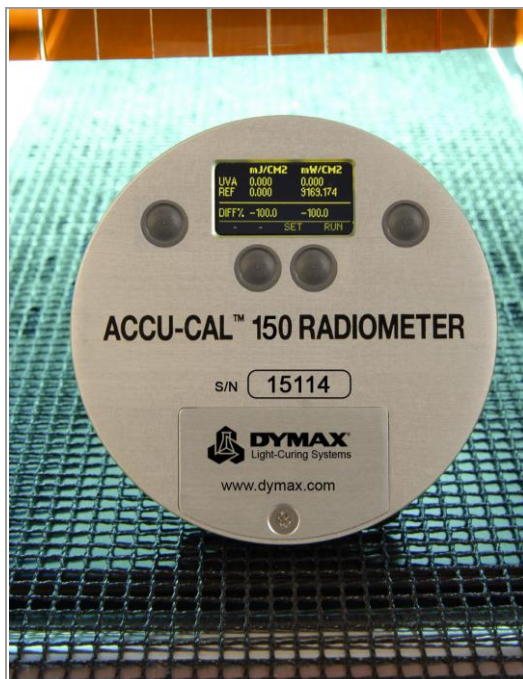
ACCU-CAL 150 for measuring UV light emitted from UV light-curing flood lamps and conveyor systems only (PN 40550)
