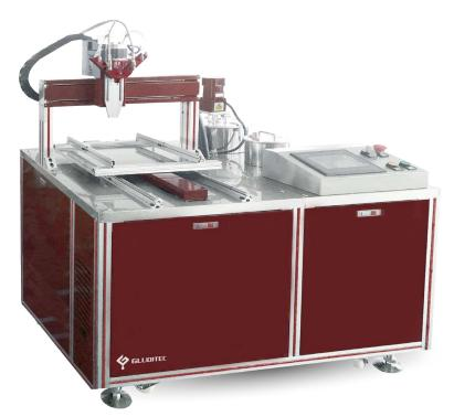
Vacuum Potting System GLT VPE-220 is a budget-friendly vacuum dispenser with advantages in bubble-free potting of small workpieces. This system is also designed in small and area-saving sizes which is just 1000 x 850 mm. GLT VPE-220 is also integrated a 3D desktop robot which helps customers easily and automatically control the precision of dispensing area.
