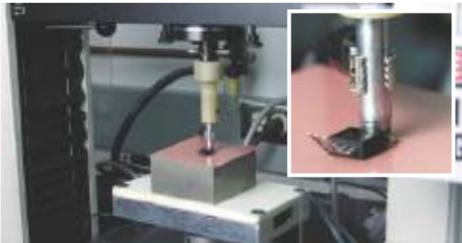
Cut-Through Resistance – The TO-220 cut-through helps customers better understand typical application performance.
