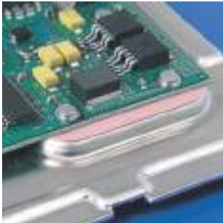
Here, BERGQUIST® SIL PAD® TSP 1600S enhances the thermal transfer from this FR-4 circuit board with thermal vias to the metal base plate.
