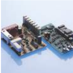
These SIL PAD® applications show clip mounting of transistors on the left and screw mounting to an aluminum bracket on the right.
