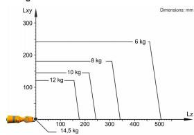
The KR 12 R1810-2 is designed for a rated payload of 12 kg in order to optimize the dynamic performance of the robot. The maximum payload of 14.5 kg applies only if the position of the center of mass is 0 mm and a supplementary load optimized for the load case is mounted. The specific load case must be verified using KUKA.Load or KUKA Compose. For further consultation, please contact KUKA Support.
