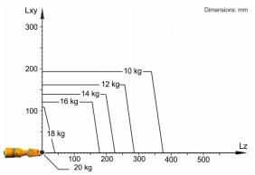
The KR 16 R1610-2 is designed for a rated payload of 16 kg in order to optimize the dynamic performance of the robot. The maximum payload of 20 kg applies only if the position of the center of mass is 0 mm and a supplementary load optimized for the load case is mounted. The specific load case must be verified using KUKA.Load or KUKA Compose. For further consultation, please contact KUKA Support.
