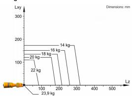
The KR 20 R1810-2 is designed for a rated payload of 20 kg in order to optimize the dynamic performance of the robot. The maximum payload of 23.9 kg applies only if the position of the center of mass is 0 mm and a supplementary load optimized for the load case is mounted. The specific load case must be verified using KUKA.Load or KUKA Compose. For further consultation, please contact KUKA Support.
