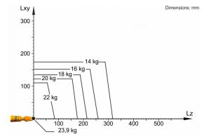
The KR 20 R1810 is designed for a rated payload of 20 kg in order to optimize the dynamic performance of the robot. With reduced load center distances, higher loads up to the maximum payload may be used. The specific load case must be verified using KUKA.Load. For further consultation, please contact KUKA Support.
