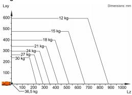
The KR 30 R2100 is designed for a rated payload of 30 kg in order to optimize the dynamic performance of the robot. The maximum payload of 36.5 kg applies only if the position of the center of mass is 0 mm and a supplementary load optimized for the load case is mounted. The specific load case must be verified using KUKA.Load or KUKA Compose. For further consultation, please contact KUKA Support.
