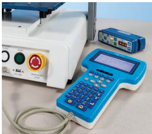
Teach Pendant simplifies setup and programming with EFD's proprietary dispensing software.
