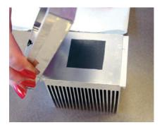
BERGQUIST® TGR 1500A is a high performance, thermally conductive compound intended for use as a thermal interface material between a high-end computer processor and a heat sink. Other high watt density applications will also benefit from the extremely low thermal impedance of BERGQUIST® TGR 1500A.
